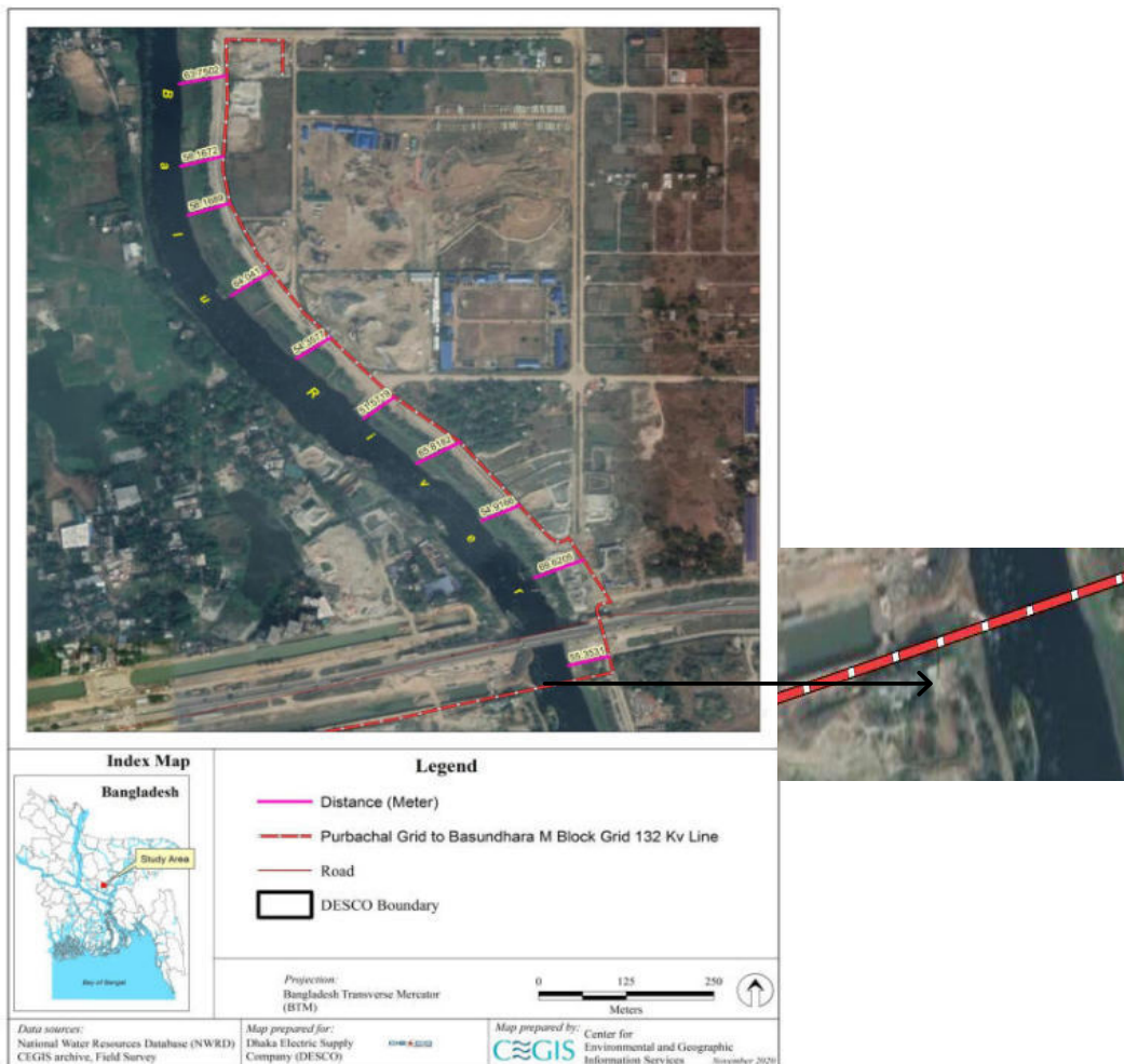
Figure 5.37: Balu River Crossing
